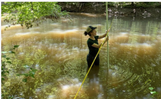
Erin Hecht, Sr. Program Coordinator, taking depth measurements along a cross-section of the creek to create a profile of the stream bed.
