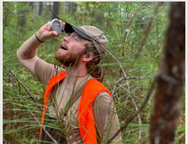
Eddie using a clinometer to measure the height of trees, an essential skill in the field of forestry.
